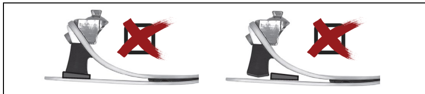
Improper Wedge Placement
